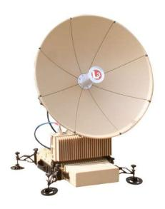
The Panther VSAT from L-3 GCS provides high-speed data communications for Internet, VPN connectivity and video transmission. This highly rugged VSAT manpack is light-weight, highly portable and offers simplistic pointing, fine-tune adjustments and control capabilities via visual indicators on the front panel and an embedded, web-based GUI. This allows for easy, accurate, and quick acquisition without bulky motors, drive systems or complex test equipment.
