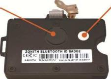
HANDLE Handle for clasp or lanyard when worn horisontally. LED Indicating: - Normal operation - Alarm status
