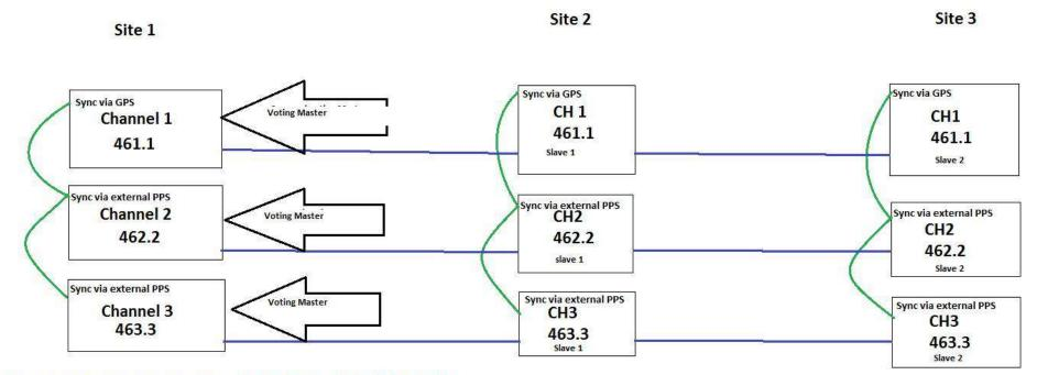
Blue lines are network connections. Green lines are PPS ribbon cables.
