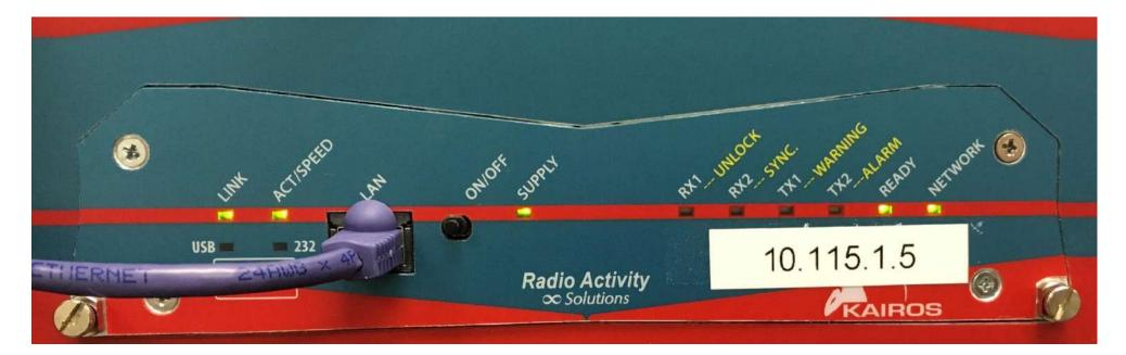
An RX1 LED that is blinking Green means the internal timing sync is satisfied.
