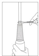
To mount the whip section it is recommended that only one section of the whip is screwed onto the antenna at a time. The whip section should be hand tightened fully then a suitable tool (ie: a spanner) can be used to tighten the section a further 10 to 20 degrees clockwise while holding the antenna body with a free hand.
