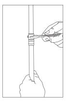
To mount 2 whip sections together the unattached whip section should be hand tightened fully then a suitable tool (ie: a spanner) can be used to tighten the section a further 10 to 20 degrees clockwise while holding the already screwed on whip section with a free hand.
