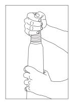
The base spring should only ever be hand tightened, if a tool is used it may damage the spring base.
