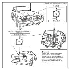
Caution:- Whilst the Barrett 2019 automatic tuning mobile HF antenna is designed to withstand vibration to military specifications on tyred vehicles, some mounting positions on large prime-movers, particularly front mounted bull bars, are subject to vibration that far exceeds this specification. Do not mount the Barrett 2019 antenna in positions such as these as damage to the antenna may result.
