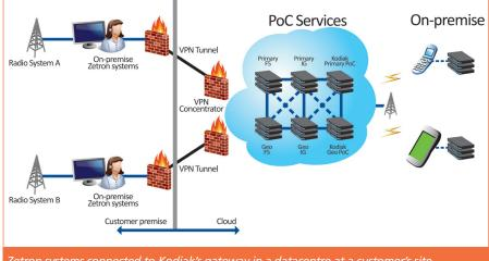
Zetron systems connected to Kodiak's gateway in a datacentre at a customer's site
